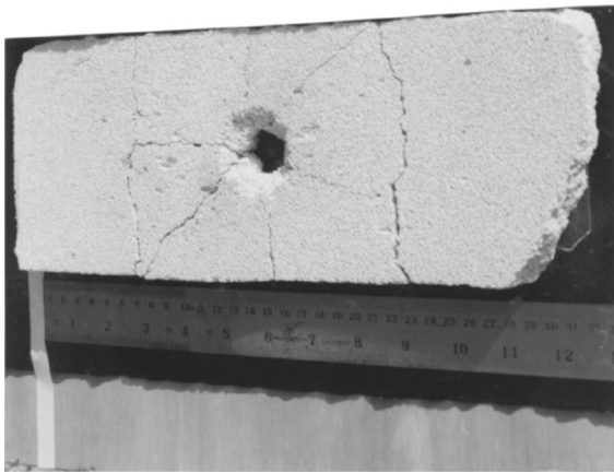
Fig. 4. Typical cracking patterns.
