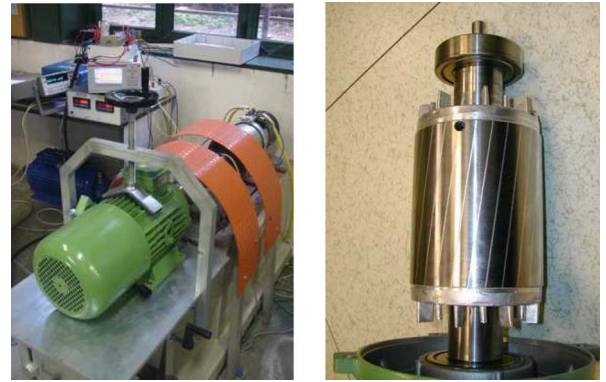
Fig. 10. Photos of the (left) test bed and of the (right) drilled rotor bar.
